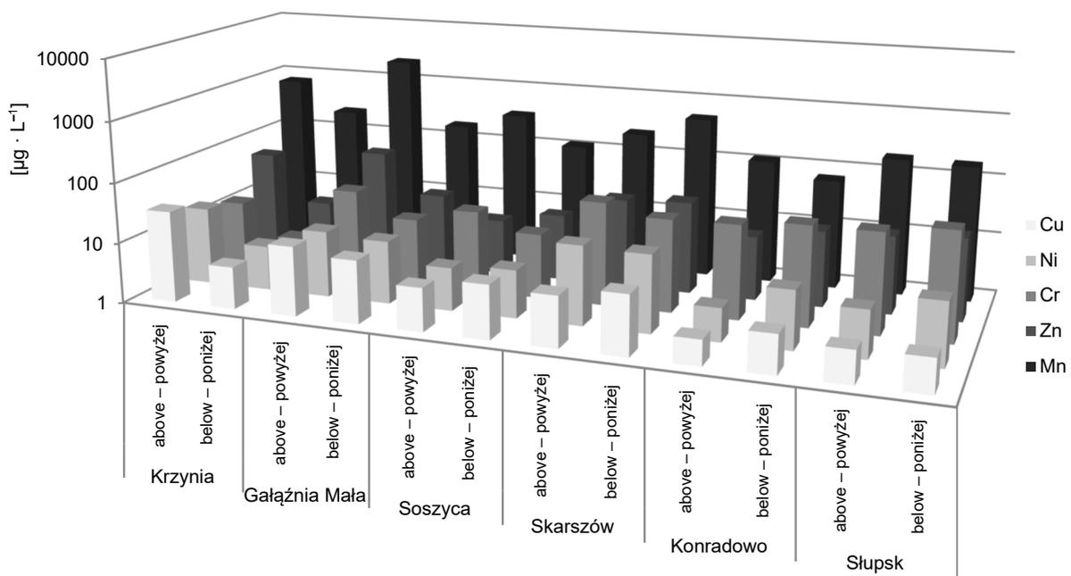
Fig. 3. Concentration of Cu, Ni, Cr, Zn and Mn in bottom sediment samples collected above and below dams of six SMPPs in the Stupia river basin
