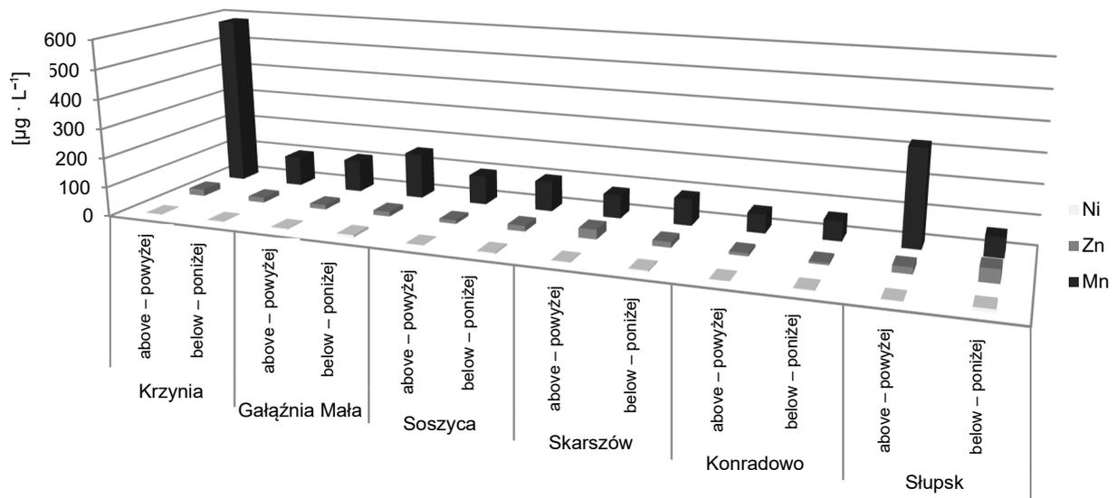
Fig. 2. Average concentration of Ni, Zn and Mn in water samples collected above and below dams of six SMPPs in the Stupia river basin
