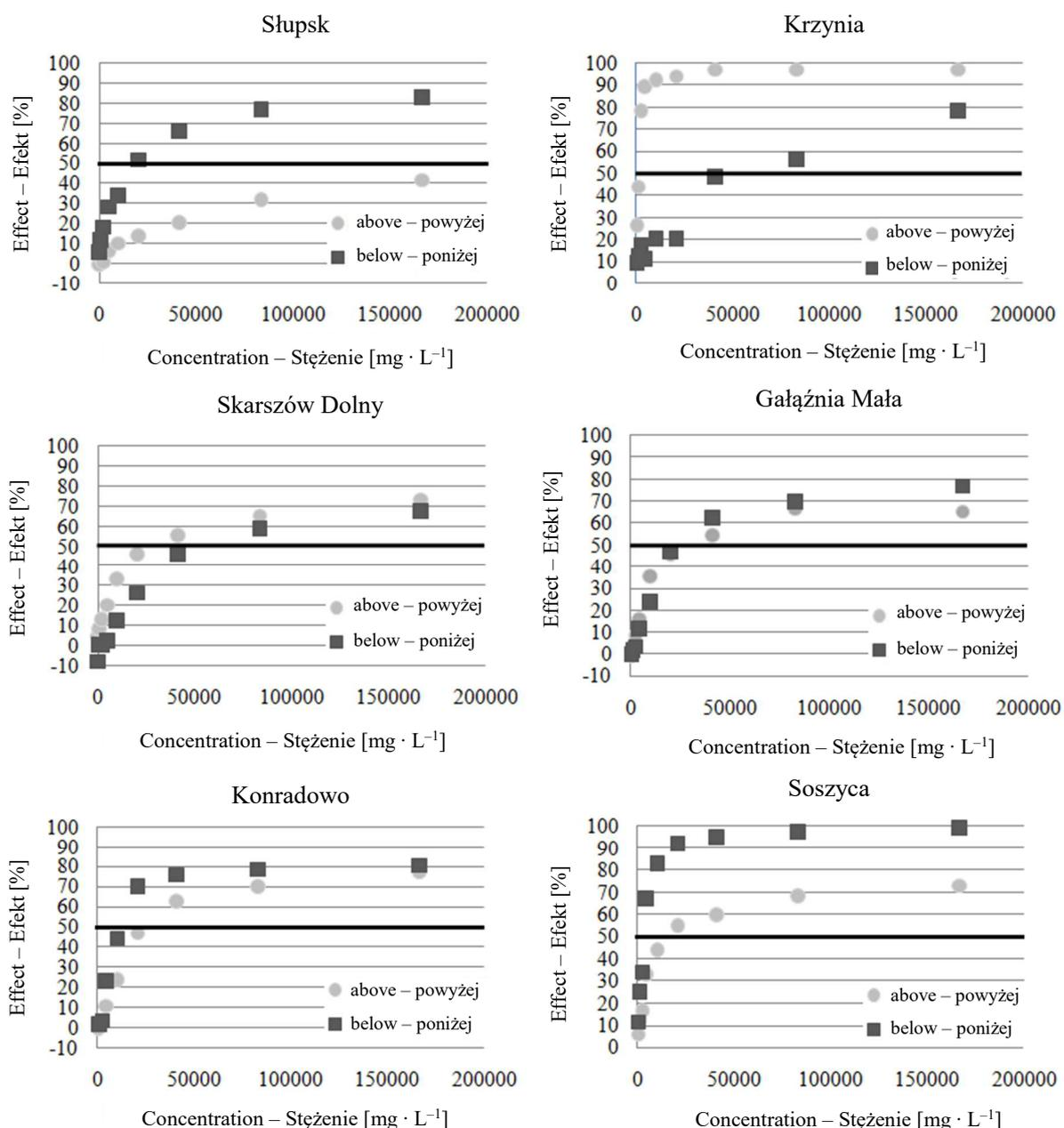
Fig. 4. Toxicity of bottom sediment samples collected above and below dams of six SMPPs in the Słupia River basin
