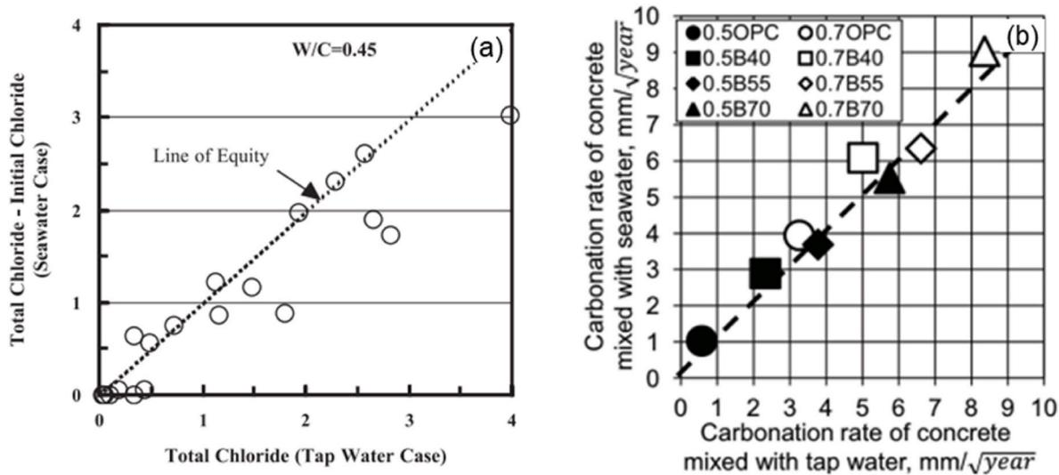
Fig. 7. Effect of seawater mixing on (a) chloride [66] and (b) carbonation ingress of concretes [79] Reproduced with permission of Elsevier, 2023.
