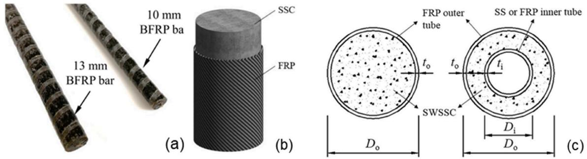
Fig. 8. FRP (a) bars (b) wraps; (c) Tubes/confinement [124–126], reproduced with permission from Elsevier 2023.
