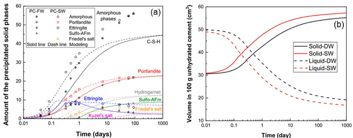
Fig. 4. Evolution of hydrated phases of cement mixed with seawater and freshwater [33]. Reproduced with permission of Elsevier, 2023.
