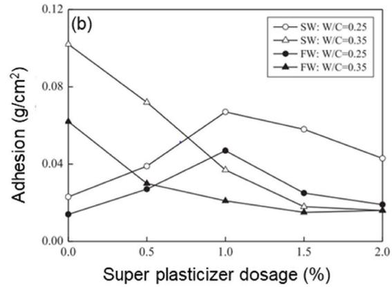
Fig. 5. Influence of seawater-mixing on fresh and rheological properties (a) [47–50] and the role of superplasticizer dosage on paste adhesion (b) Reproduced with permission of Elsevier, 2023 [48].
