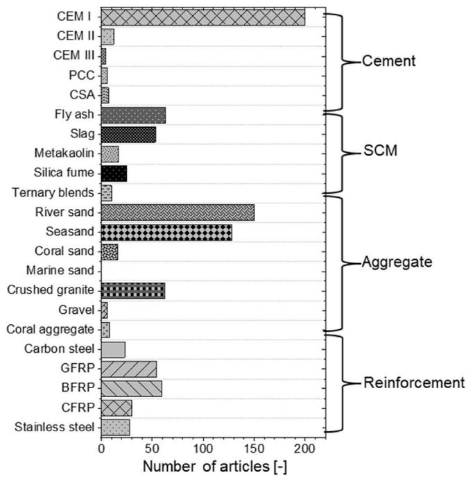
Fig. 2. Raw materials used in SW-SS concretes according to the available literature.
