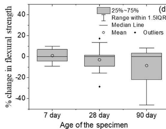
Fig. 6. Effects of seawater mixing on the mechanical properties of concrete: % change in compressive strength – (a) Age of specimen; (b) Binder type; (c) % change in Elastic modulus; (d) % change in flexural strength [55,57–66].
