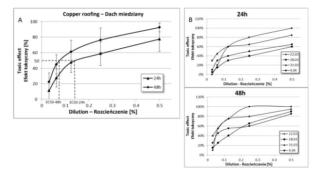
Fig. 2. Toxicity of runoff from copper roof coverage. A – means for four rain events, B – toxic effect plots for each rain event for 24 (up) and 48 (down) hours of exposure of the test organisms on the rooftop wastewater
