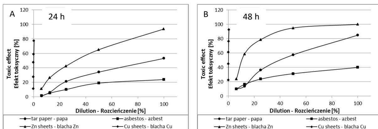
Fig. 1. Graphs of rainwater runoff toxicity from the roofs of varying coverage for 24 (A) and 48 (B) hours of exposure of the test organisms on the rooftop wastewater
